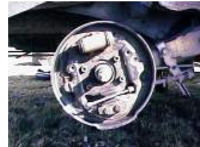
Remove parking brake cable
